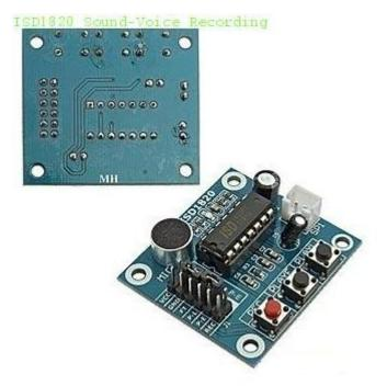
Product Description: First, the main chip: ISD1820 Second, the size: 38mm \* 42.5mm Third, the working voltage: DC 3-5V Fourth, the main features:
